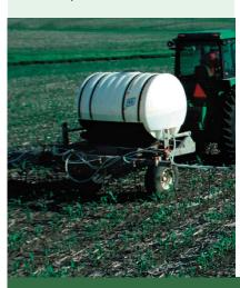
Calibration is the process of measuring application rates of your sprayer based on speed, pressure, nozzle size/type, or a combination of the three. All sprayers, including hand held, back pack, and boom sprayers should be calibrated several times during the growing season or whenever you change chemicals.
